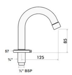
Model TVS6913 is our deck mounted basin spout for use with our knee operated time flow valve. Modern fixed design.
